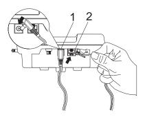
2. Place the power cord in the left molded channel on the bottom of the Base Unit.
